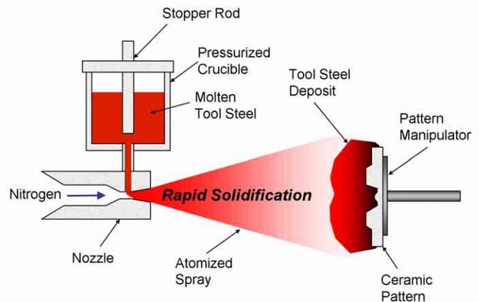
After spraying, the metal is cooled to room temperature and separated from the pattern. The irregular periphery, or overspray, of the freshly sprayed tool is squared off either by machining or, in the case of harder tool steels such as H13, by wire EDM [4]. The squared-off insert is then fixed to a mold base. Injection molds or die-cast molds require two inserts, one for each mold half.
