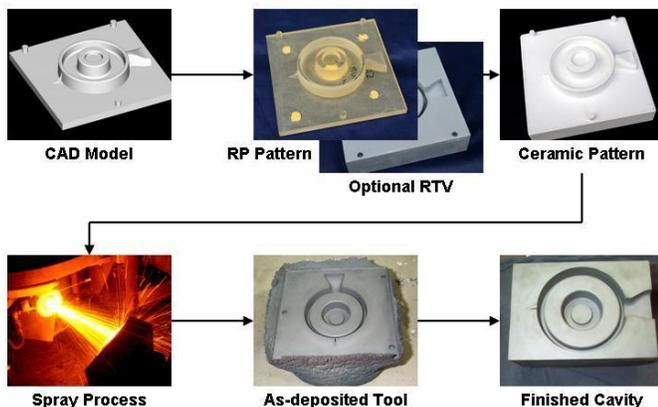
Once the mold is created, metal alloy with the desired chemistry (in cast, forged, powder or scrap form) is melted in a crucible and then injected into a nozzle with a flowing gas stream. The high velocity inert gas jet generates molten metal droplets, on the order of 50 microns in diameter, which are sprayed onto the ceramic pattern, replicating the pattern's contours, surface texture, and details (Figure 2.2).
