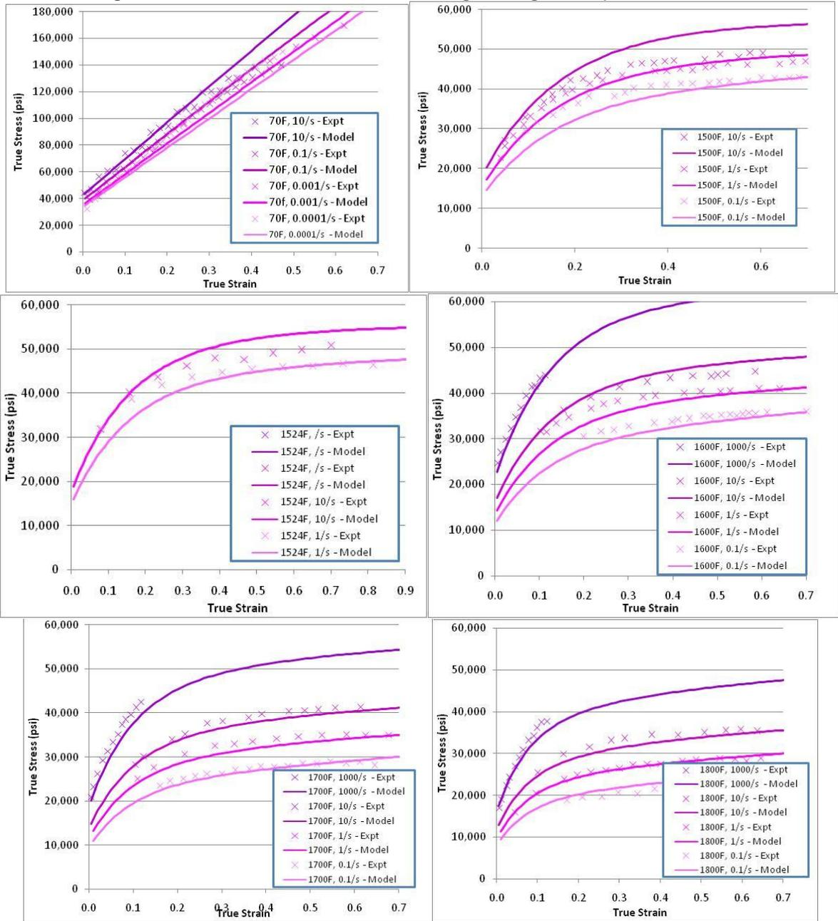
Figure 2. Stress-strain data from two-stage compression tests.
