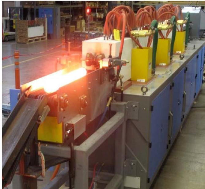
Figure 1. InductoForge™ system for heating billets or bars.
