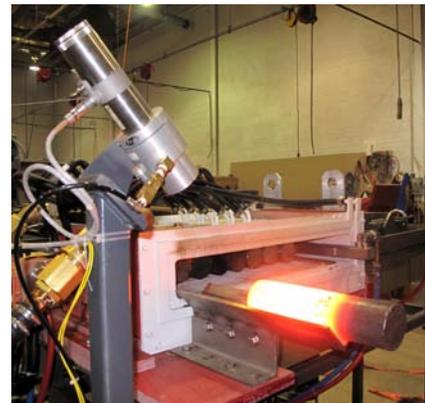
Figure 3. Various coil design can be used to provide selective heating.
