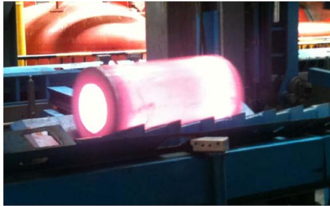
Figure 2. In some cases, the initial temperature of the workpiece prior to induction heating is considerably non-uniform.
