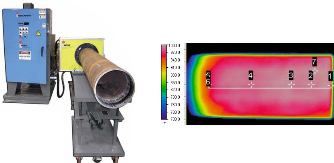
Figure 4. FluxManager™ Technology (US Patent No. 7,317,177) to stress relieving of steel tube/pipe ends.
