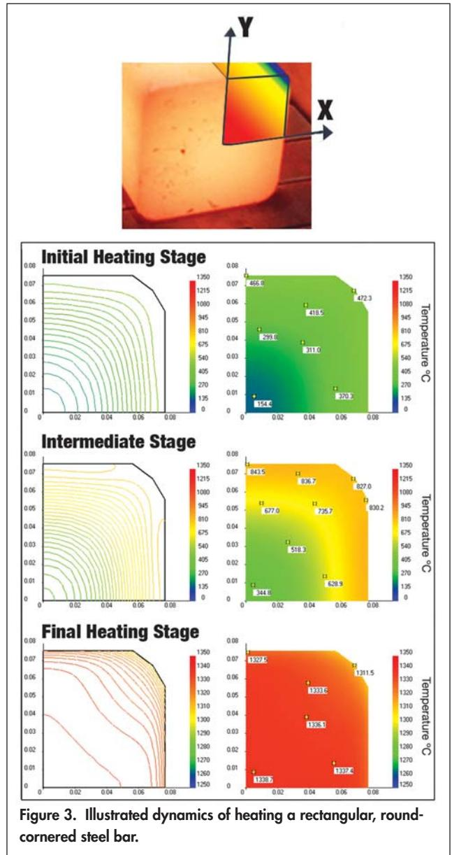
cornered carbon-steel bar of 0.1-meter (4-inch) cross section using a frequency of 500Hz. Significant temperature gradients occur within the bar cross section. It is important to have a clear understanding of the magnitude of these gradients during initial and intermediate heating stages. With intensive heating, longitudinal and transverse cracks may occur as a result of significant thermal stresses caused by different magnitudes of temperature and temperature gradients.
