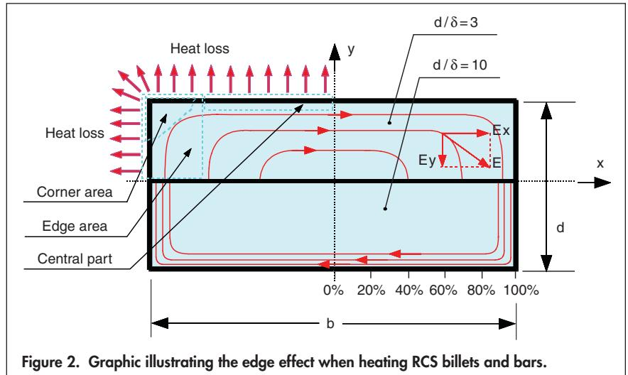
Figure 2. Graphic illustrating the edge effect when heating RCS billets and bars.
