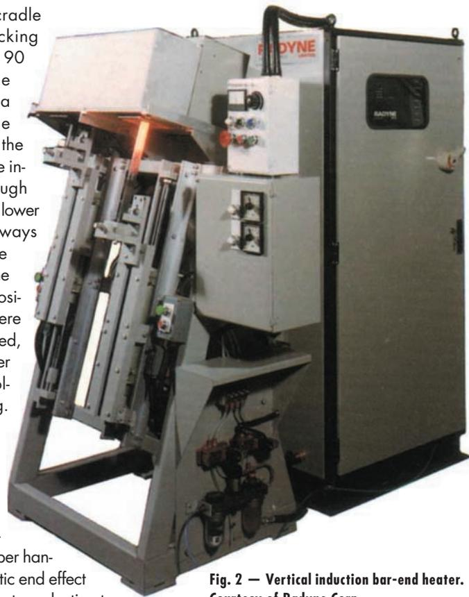
Fig. 2 — Vertical induction bar-end heater. Courtesy of Radyne Corp.
