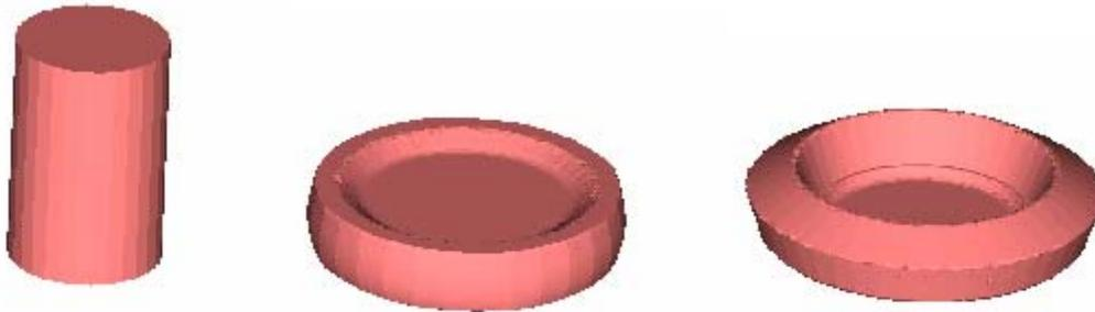
Figure 7: Initial, intermediate, and final shapes of the forging process
