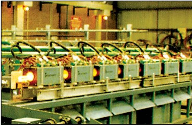
**FIGURE 3: In-line induction steel bar heater**
