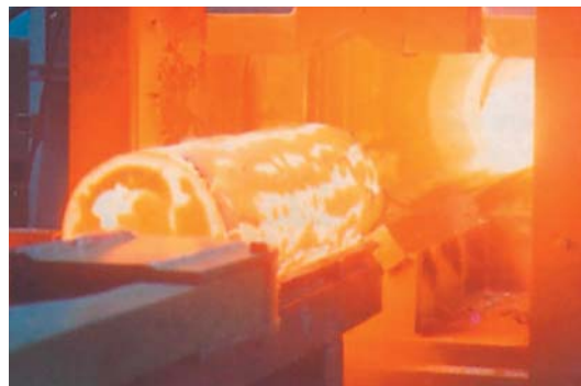
Fig. 1 — Progressive multistage horizontal heating of large steel billets.
