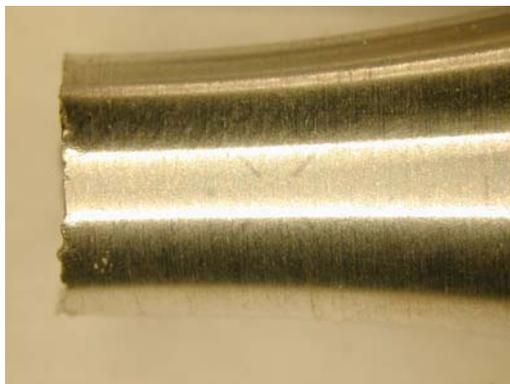
**Figure 15: Photo of the polished surface of a fatigue specimen (in the neck region). This sample had been tested and the fracture is on the left side of the photo.**
