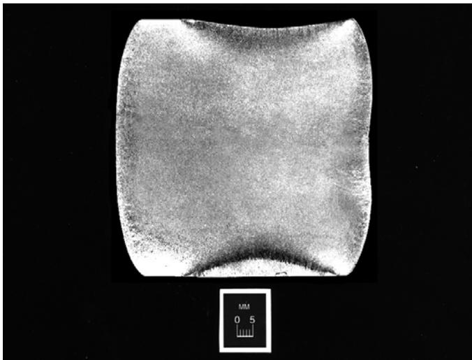
**Figure 3: Longitudinal macro-structure of AA2618 billet after upsetting 50% at 427C (800F). The grain structure remained similar to that of the as-extruded condition. Pre-heating of this sample was via conventional methods. Extrusion and forging directions are vertical to the page. Photo was taken at ORNL.<sup>13</sup>**
