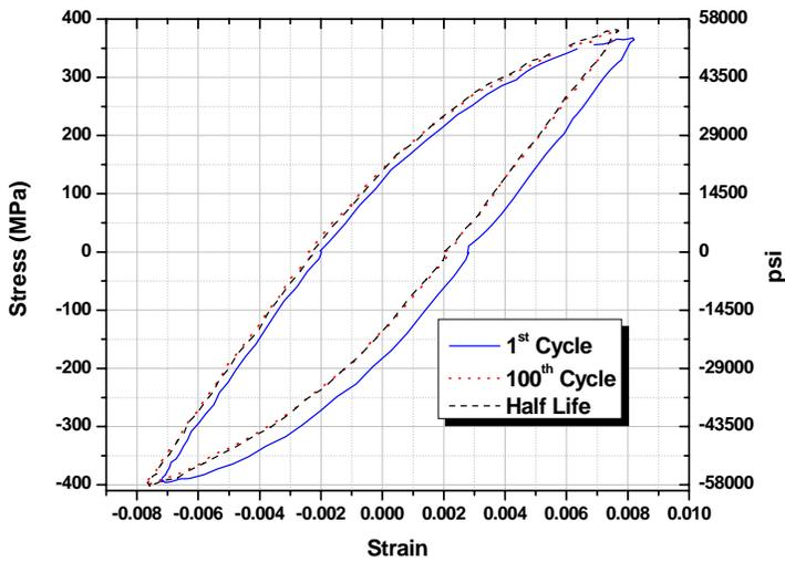
Figure 17: Hysteresis of strain controlled, low cycle fatigue testing. Data were for an IR solutionized sample (20 min @ 539 C).
