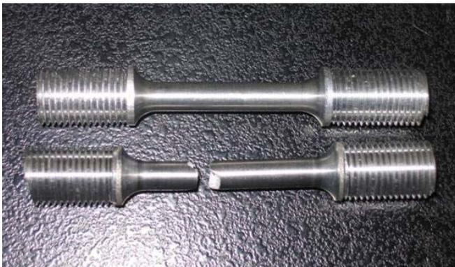
Figure 18: AA2618 LCF samples before and after testing.
