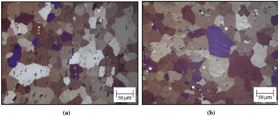
**Figure 21: Micro-graphs showing the grain size in (a) an IR solution treated sample (530 C for 40 min) after ageing, and (b) a sample that was conventionally solution treated and aged. The section shown in (a) is parallel to the forging direction and the section in (b) is transverse to the forging and extrusion directions.**
