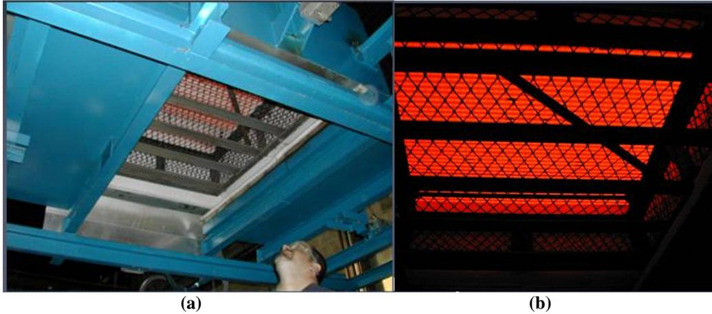
**Figure 5: Photographs showing the “underside” of the prototype production IR drop furnace installed at the Queen City Forging Company. The photos show the steel-mesh basket in which the parts are place for heat-treating. The parts-basket drops into a quench tank after solution treatment. Photo courtesy of QCF.**
