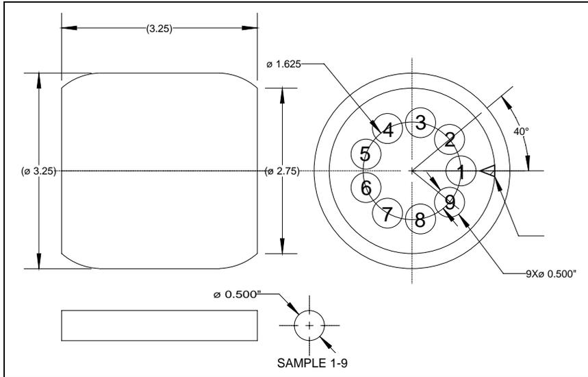
**Figure 9: Sample layout with respect to forging upset. Samples from IR heat-treated upsets were produced in this manner.**
