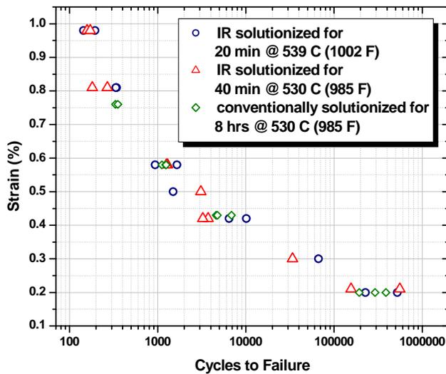
Figure 20: Low cycle fatigue data for conventionally heat-treated and rapid IR treated samples.
