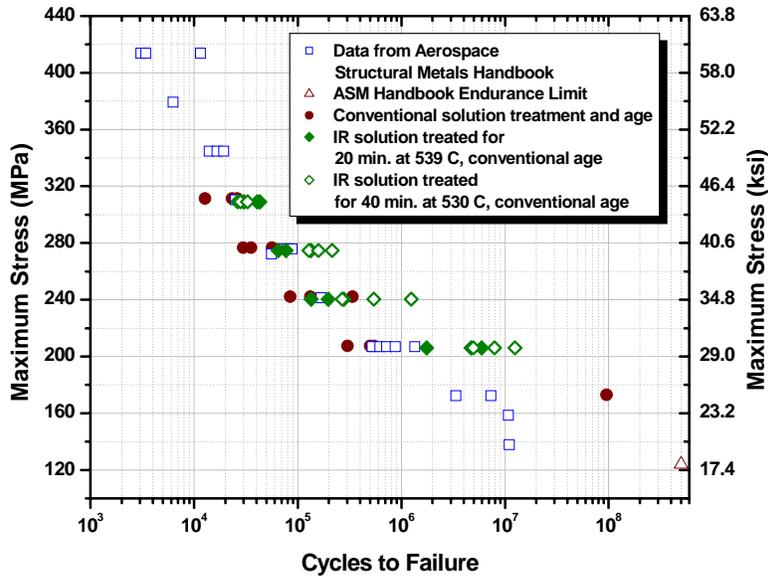
Figure 19: High cycle fatigue data. Graph shows a comparison of high-cycle fatigue data for T61 treated specimens that were conventionally solution treated, IR solution treated and data from the Aerospace Structural Metals Handbook.<sup>22</sup>
