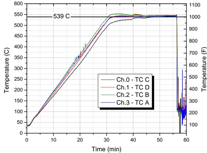
**Figure 7: IR furnace solutionizing thermal cycle data for AA 2618 forged upsets. Target thermal profile was for 20 minute soak time at 539 C (1002 F). Thermocouples were imbedded in the center of the forged upsets.**
