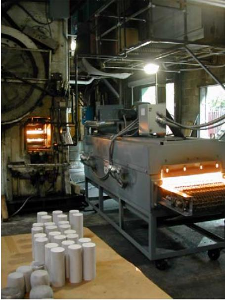
**Figure 2: Continuous flatbed IR furnace (right) and forging billet (left-foreground) at the Queen City Forging Company. The forging press with die heater is shown in the background. Photo courtesy of QCF.**
