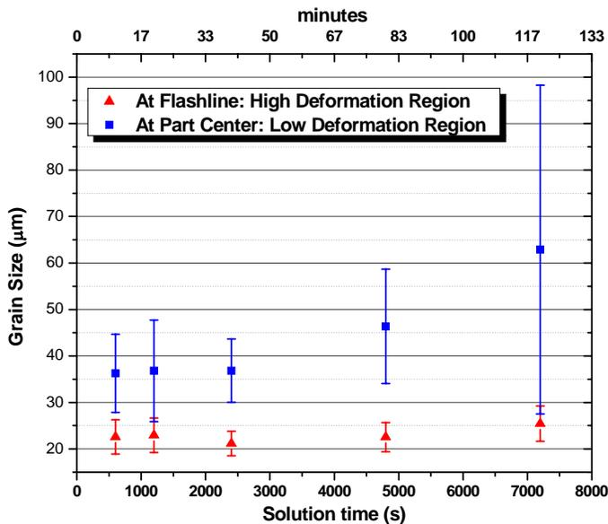
Figure 23: Variation of grain size in forged and IR solution treated prototype parts. Error bars represent  $\pm 1$  standard deviation.<sup>26</sup>
