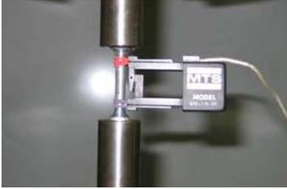
Figure 16: LCF test configuration.
