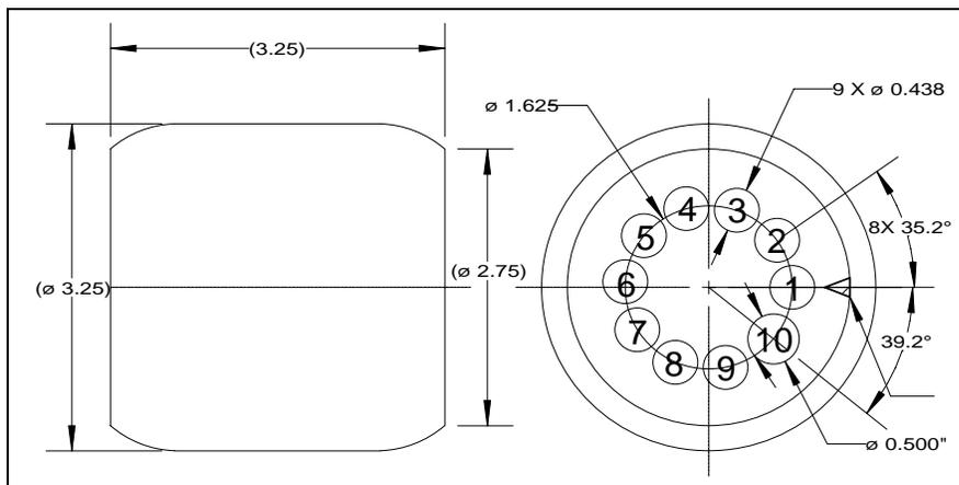
**Figure 8: Sample layout with respect to forging upset. Samples from conventionally heat-treated upsets were produced in this manner.**
