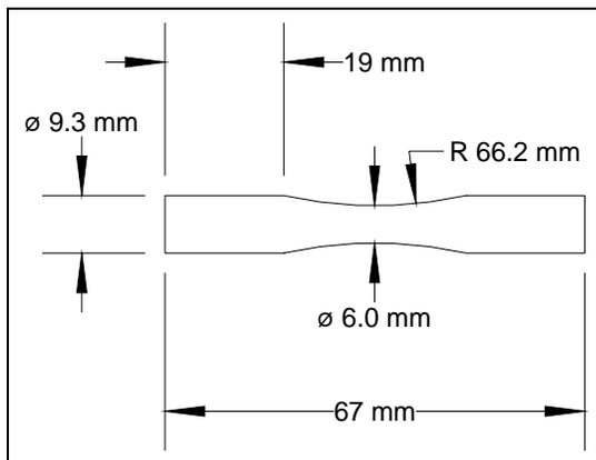
**Figure 14: Sketch of HCF R.R. Moore fatigue specimens used for this study.**
