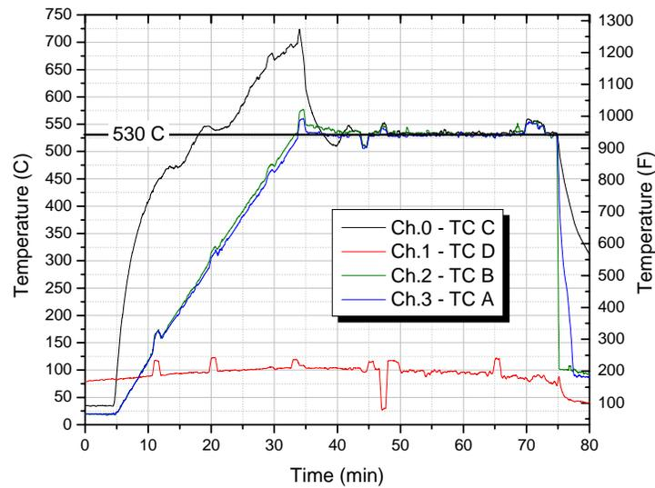
**Figure 6: IR furnace solutionizing data for AA 2618 forged upsets. Thermocouples were imbedded in the center of the forged upsets. Target thermal profile was for 40 minute soak time at 530 C (985 F). Ch.0 is the furnace temperature and Ch.1 is the quench bath temperature. Sharp/fast spikes in the data are due to excessive noise that was not filtered from the data.**
