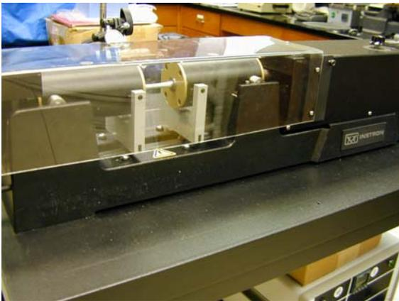
**Figure 12: Photograph of Instron, R.R. Moore fatigue testing machine.**
