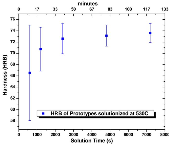
Figure 22: Hardness in forged and IR solution treated prototype parts as a function of time at temperature. Parts were given a conventional artificial ageing cycle. Error bars represent  $\pm 1$  standard deviation.<sup>25</sup>
