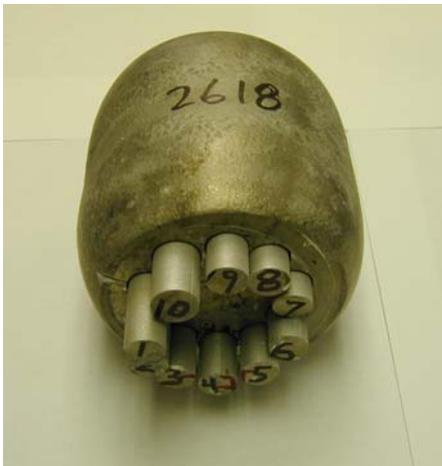
**Figure 10: Photo shows rods that have been wire-EDM machined from an AA 2618 forging upset that was conventionally heat treated. Rod samples were further machined into samples for tensile testing, and low and high cycle fatigue testing.**
