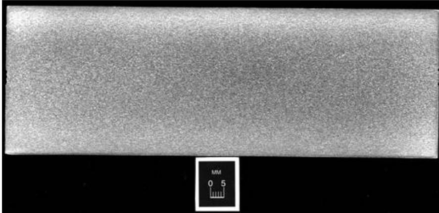
**Figure 1: Longitudinal macro-structure of AA 2618 forging billet in the as-extruded condition. The photo shows a fine, recrystallized grain structure. Extrusion direction is horizontal to page. Photo was taken at ORNL.<sup>12</sup>**
