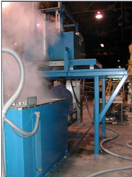
**Figure 4: Photograph of the prototype production IR drop furnace installed at the Queen City Forging Company. The IR furnace elements are located in the top-middle unit, and the quench bath (from which the steam is rising) is shown at the bottom-left. Photo courtesy of QCF.**
