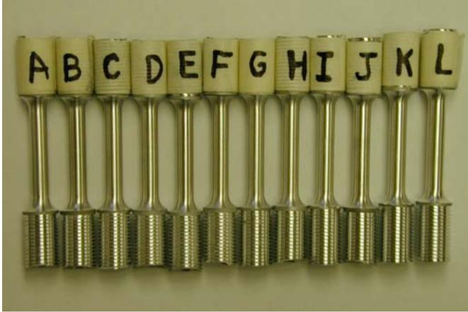
**Figure 11: Tensile test specimens CNC machined from ½” diameter rods. One specimen from each forging upset was produced.**
