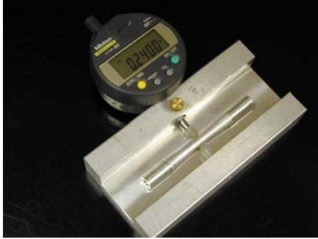
**Figure 13: Special gauge made to measure the diameter of fatigue specimens. The anvils are made of nylon so as not to damage the polished surface of the specimen.**
