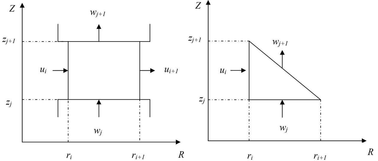
Figure 1. Boundary velocities for rectangular and triangular elements
