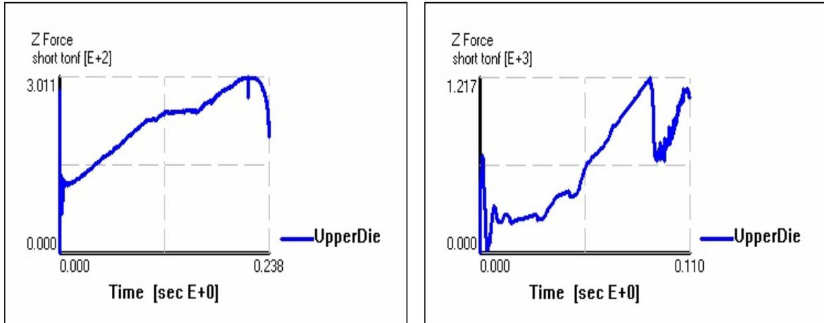
Figure 6. Die load vs Time for stage 1 and stage 2
