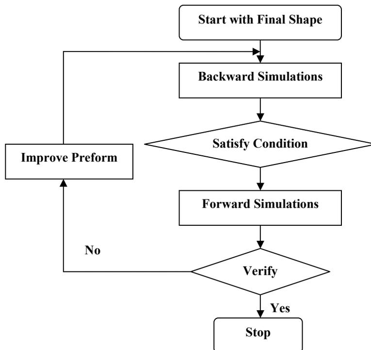
Figure 3. Flow chart of the forging preform design process
