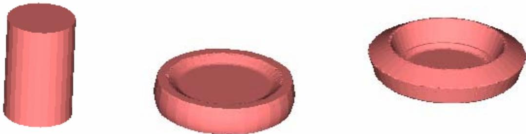
Figure 5. Initial, intermediate, and final shapes of the forging process
