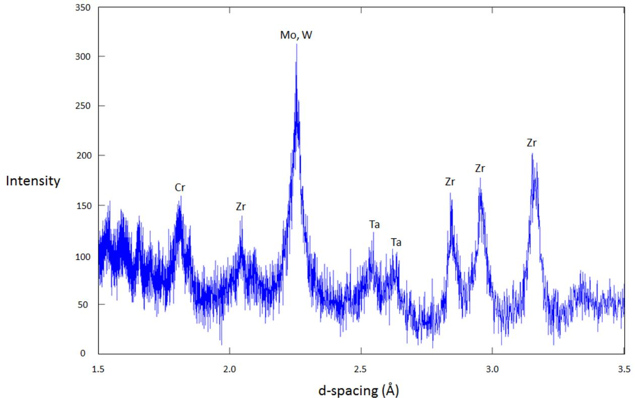
**Figure 5.** XRD plot of intensity versus d-spacing of the 1100 W clad CrMoTaWZr HEA on a H13 die head sample.
