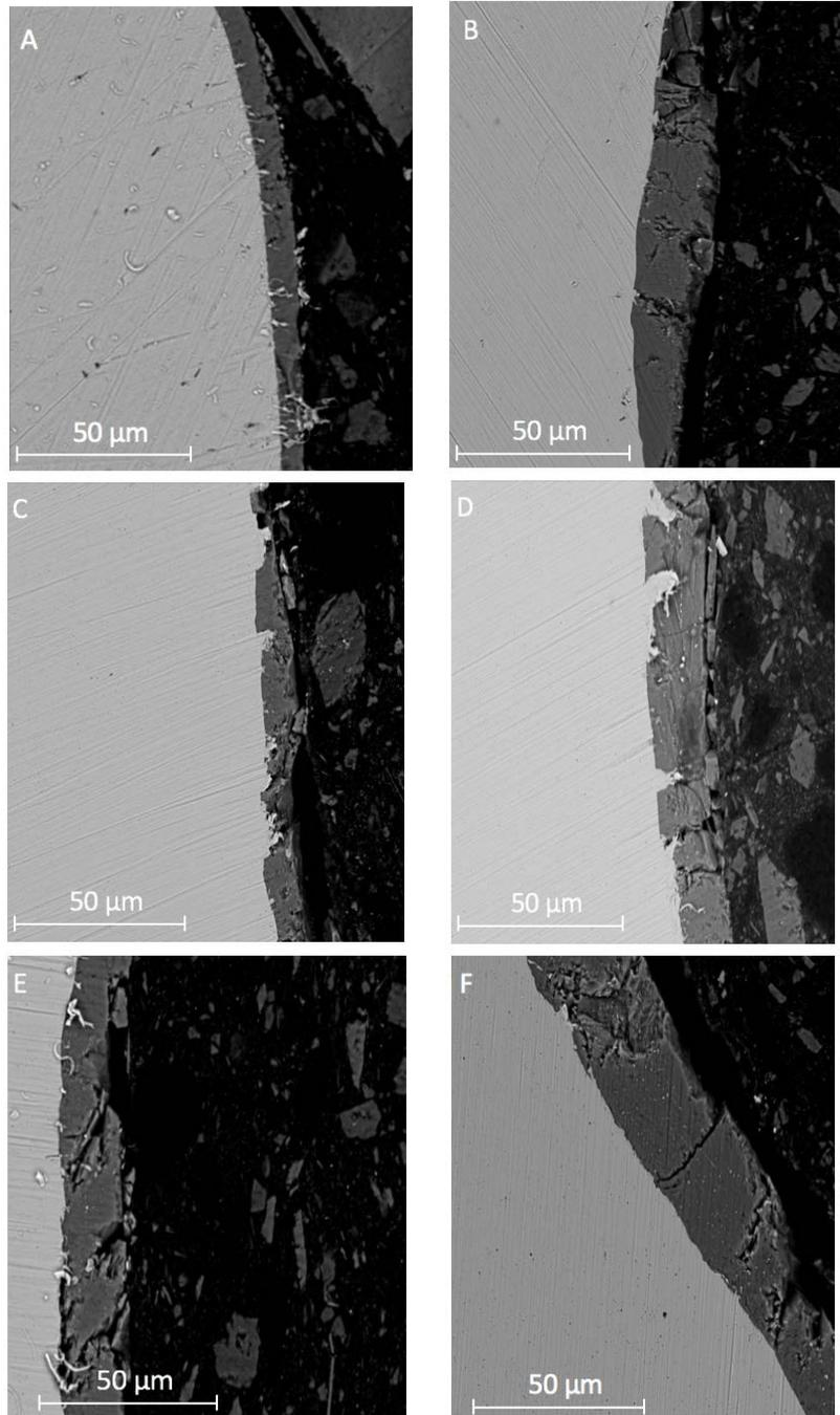
**Figure 6.** SEM images of the cross-section (first column) and close-up (second column) of a laser clad  $\text{Al}_{3.3}\text{Co}_{24.2}\text{Cr}_{16.1}\text{Fe}_{16.1}\text{Ni}_{24.2}\text{Ti}_{16}$  HEA on a H13 die head sample corresponding to eight different power settings: A (500 W), B (600 W), C (700W), D (800 W), E (900 W) and F (1000 W)
