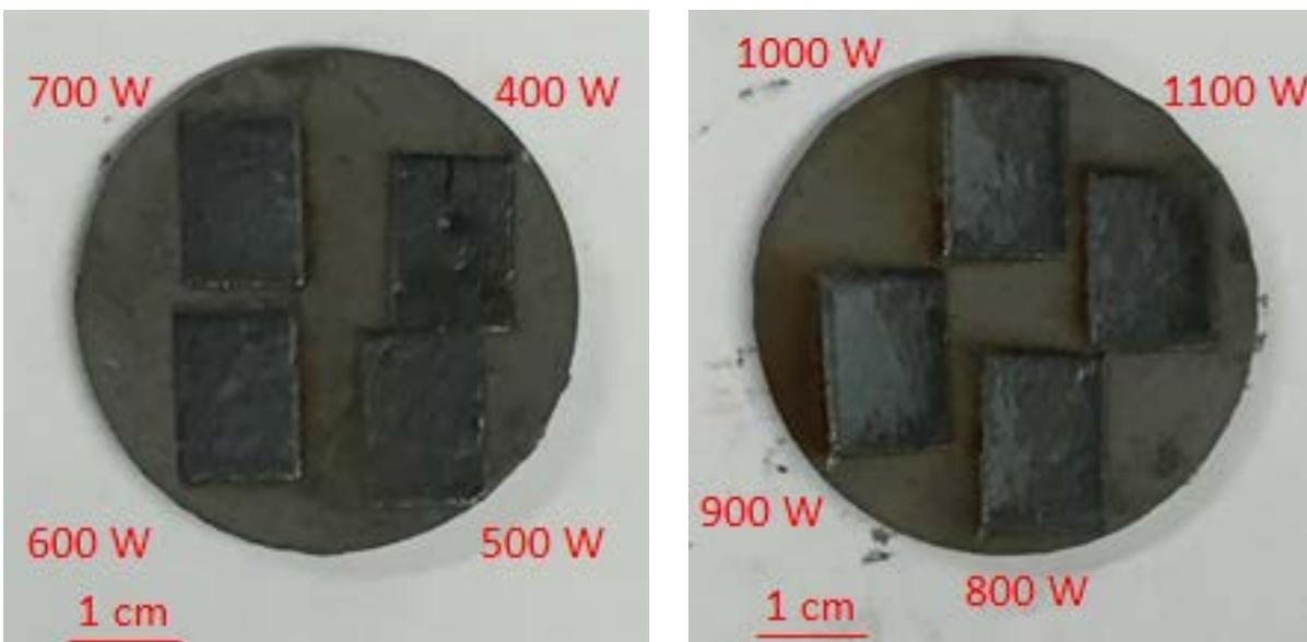
**Figure 3.** Optical images of H13 steel samples from a die head showing squares where  $\text{Al}_{3.3}\text{Co}_{24.2}\text{Cr}_{16.1}\text{Fe}_{16.1}\text{Ni}_{24.2}\text{Ti}_{16.1}$  HEA has been laser clad to the surface at eight different power settings ranging from 400 W to 1100 W in increments of 100 W.
