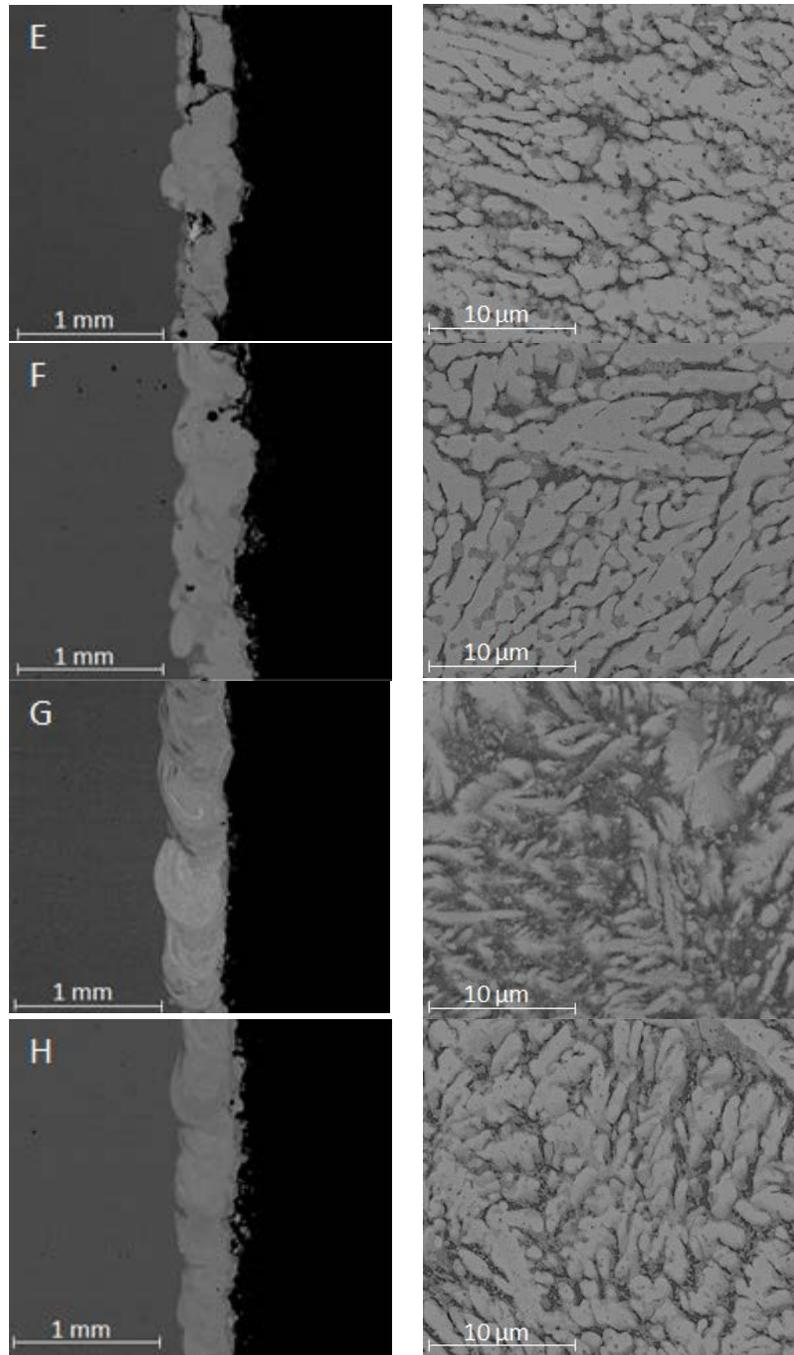
**Figure 4.** SEM images of the cross-section (first column) and close-up (second column) of a laser clad CrMoTaWZr HEA on a H13 die head sample corresponding to eight different power settings: A (400 W), B (500 W), C (600W), D (700 W), E (800 W), F (900 W), G (1000 W) and H (1100 W).
