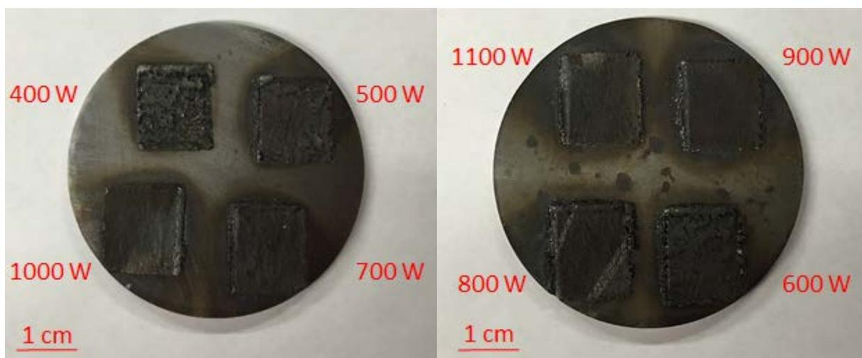
**Figure 2.** Optical images of H13 steel samples from a die head showing squares where CrMoTaWZr HEA has been laser clad to the surface at eight different power settings ranging from 400 W to 1100 W in increments of 100 W.
