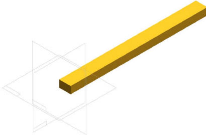
Figure 6: 1<sup>st</sup> run billet: 0.625'' x 1'' x 12'' long
