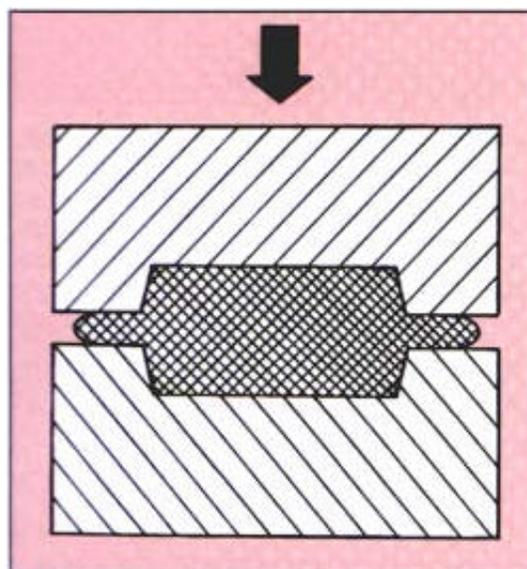
Figure 2: Impression Die Forging
