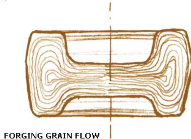
Figure 1: Forging grain structure
