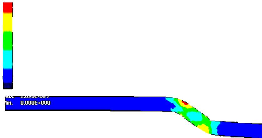
Figure 7: SuperForge results – Billet plastic strain for bending
