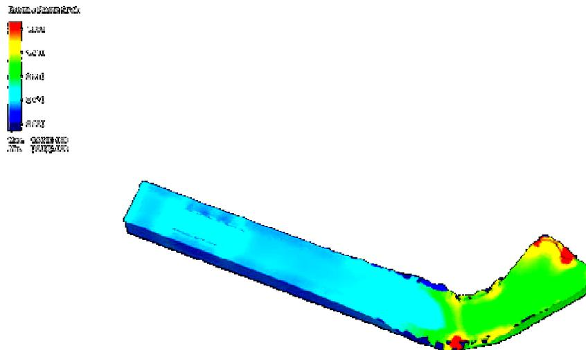
Figure 8: SuperForge results – Billet plastic strain for forging
