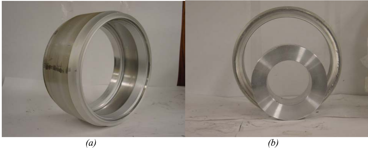
Figure 10: (a) Rings produced, (b) Compared with initial workpiece
